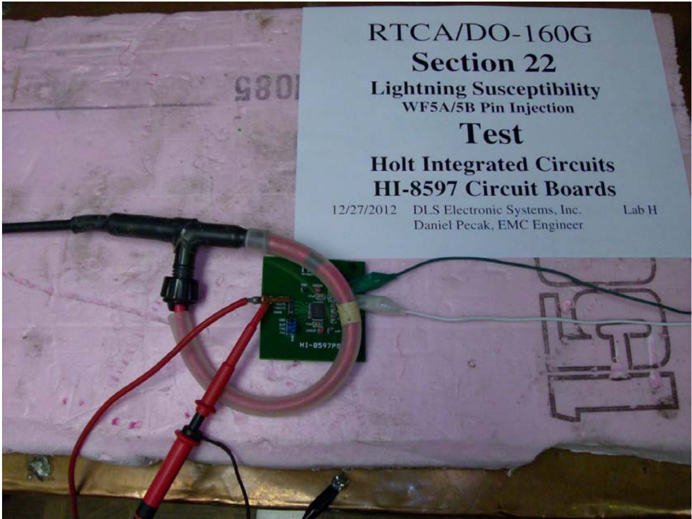
WF5A/5B Pin Injection--Test
